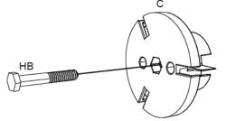
Attach the Wheel Clicker (C) to the D-Tube, and secure with the hardware shown.
