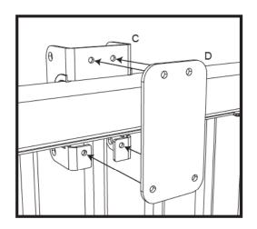
Secure the Bracket (C) and Plate (D) using the hardware shown.
