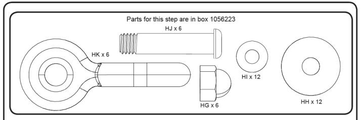
Attach the Swing hardware to the Swing Bar (A) while the Swing Bar is still on the ground. Do not over tighten.
