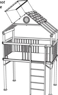
The Roof Panels (C) placed on top need to have a notch as shown.
