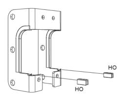
Make sure the Bracket (C) is placed on to a D-Tube with the D-Tube fitting into the opening of the Bracket as shown. Bring the Plate to the Bracket and line up the holes in the Plate (D) with the holes in the Bracket (C).
