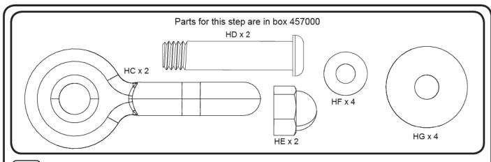
Attach the hardware shown to the Trapeze Swing Bar (A) while the Trapeze Bar is not attached to the Monkey Bars. Do not over tighten.
