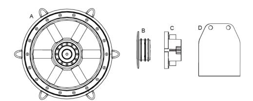
Place the Universal Bracket Cap (HG) and the Universal Bracket (D) on the D-Tube in the desired location. Twist the Universal Bracket (D) in order to get it between the Railings.
